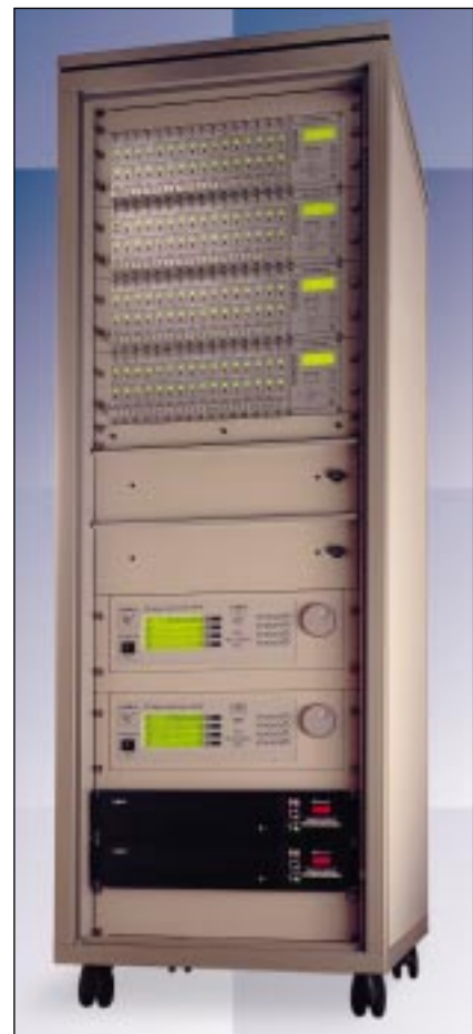
FIGURE 4. Chip-on-carrier and packaged laser diode burn-in tests are performed in rack-mounted, computer-controlled test platform that includes diode fixturing and all associated current-driver, temperature-control, and data-acquisition electronics.
